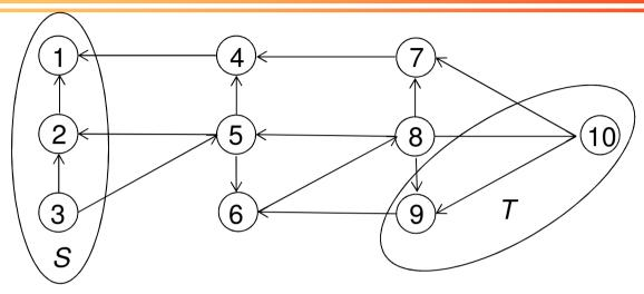
We apply the procedure *findpath(S,T)* with FIFO queue (bfs) and obtain the labels (resulting in a path with a minimum number of arcs)
