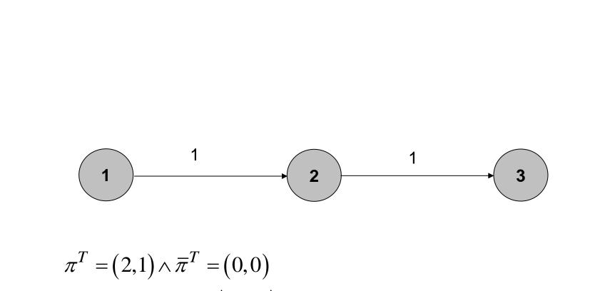
The shortest path (1, 2, 3) has an objective function value of 2.
